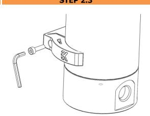
Once the reservoir is positioned please use enclosed 2.5mm Allen key to tighten the hex head screw in order to clamp the reservoir. Do not use high force. Partially unscrew the aforementioned screw when removing the reservoir.
