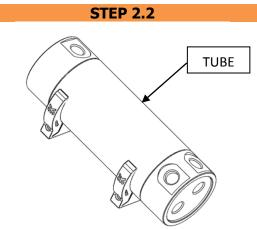
Install reservoir onto reservoir holders. Using a gentle force the reservoir will easily 'click' into position. The clamps should always hold onto acrylic tube and not the acetal top or bottom.
