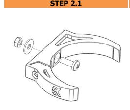
Use enclosed M4 screw, washer and nut to mount the reservoir holder through the pre-drilled hole to the computer chassis.
