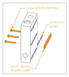
Tighten the three (3) enclosed M4x25 DIN7984 screws to EK-FC Terminal BLANK Parallel using Allen (hex) key 2.5mm.
